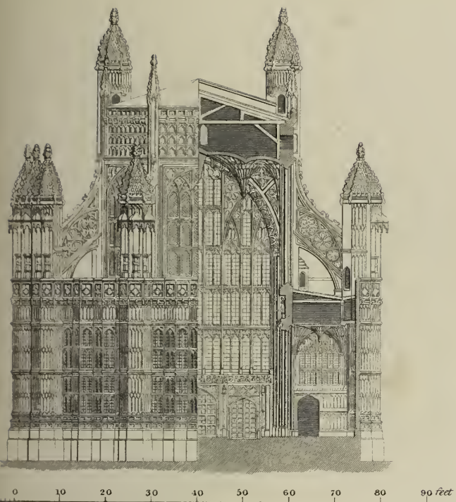
Half Elevation and Section and a Plan of Henry the Seventh's Chapel at Westminster.
